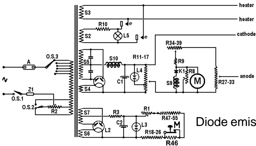
Diode emission test
