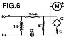
The deflection of the meter is non-linear due to the frequency dependency of K2. The cards for measuring the output power don't have a transformation scale because only the maximum of the deflection is used when adjusting a device.
