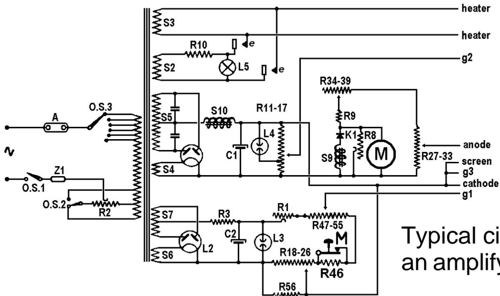
Typical circuit for testing an amplifying valve.
